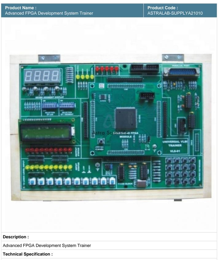
This training system consists of FPGA chip with higher logic elements and large number of pins. Therefore, students are able to develop, implement and verify design of basic or advanced digital circuit, digital signal processor and CPU/MCU.
