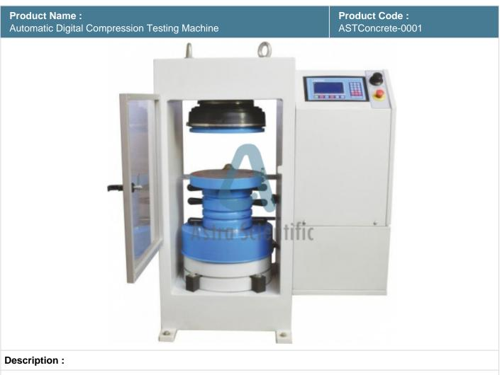
Automatic Digital Compression Testing Machine
