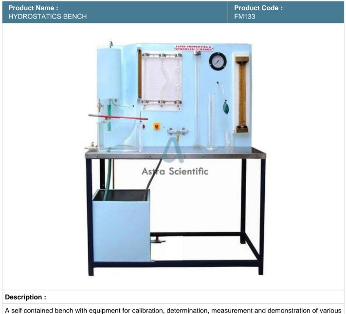
A self contained bench with equipment for calibration, determination, measurement and demonstration of various properties or behavior of fluids under static conditions. Over 15 experiments
