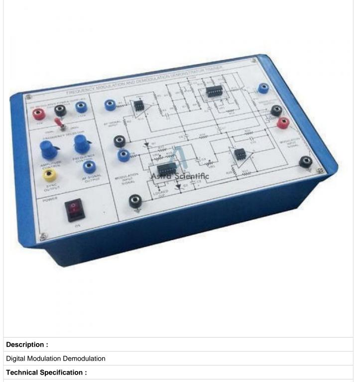
The design and construction of electron With this board the students can study the operating principle of the digital communications using the most common techniques such as PCM modulation, PAM modulation, PFM modulation, PWM and PPM modulations and finally the DM modulation with the aid also of a signal of noise, of analog filters and output amplifiers. ic circuits to solve practical problems is an essential technique in the fields of electronic engineering and computer engineering.
