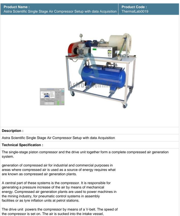
the compressor is set on. The air is sucked into the intake vessel, where it settles before it is compressed inside the compressor. The compressed air is then delivered to a pressure vessel and is available as a working medium. To set a steady flow-operating mode, the compressed air can be discharged over a blow-off valve with a silencer. A pressure switch with a solenoid valve for limiting the pressure and a safety valve complete the system.
