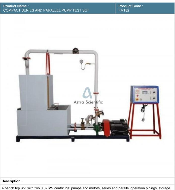
A bench top unit with two 0.37 kW centrifugal pumps and motors, series and parallel operation pipings, storage tank, and measuring instruments. Optional : Advanced inverter for speed control as well as for motor speed and output power indication.
